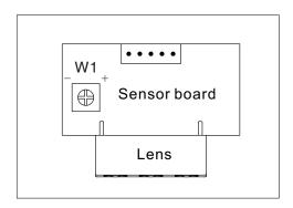
Disassembling the cover, and adjust the W1, turn clockwise to increase the distance, and counter clockwise to reduce the distance.
