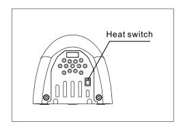
User can adjust warm or cool air according to the request. When turn on the heat switch, it will be warm air .When close the heat switch, it will be cool air.
